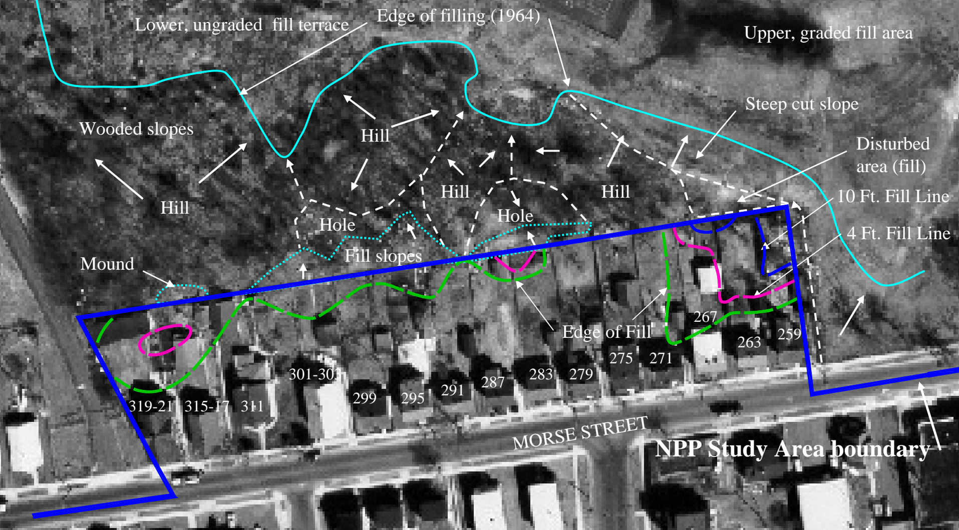
1964 aerial photograph with close-up of properties in Block A along Morse Street and wooded slopes to their north showing former topography and fill areas now covered by subsequent filling up to study area boundary line. Annotations are features visible with a stereoscope. Solid arrows point down-slope, dashed arrows are aligned with swales. Light blue outlines are fill areas visible within depressions that are now within the school athletic fields (Public Properties Study Area). Green outline is the continuation of these fill areas within backyards of these homes (Non-Public Properties Study Area) as mapped by the Initial and Supplemental investigations. Magenta and blue lines are 4 and 10-foot thick fill contour lines.
